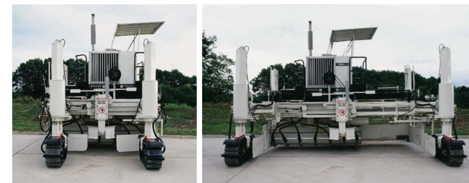
Captions Top left: SF-2 offers unique variable width capabilities. Top right: Spreading using the hydraulic plow. Above right: SF-2 features CMI Hydra-mation® grade control. Bottom left: SF-2 in transport mode. Bottom right: Transition to paving mode takes minutes and requires no added extensions.
